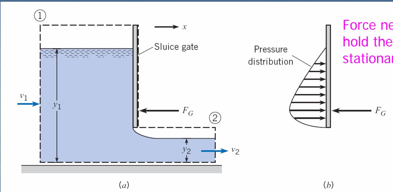
$$\bar{p}_1 A_1 = \gamma \left( \frac{y_1}{2} \right) \times (y_1 b) \quad b = \text{width of the gate}$$
