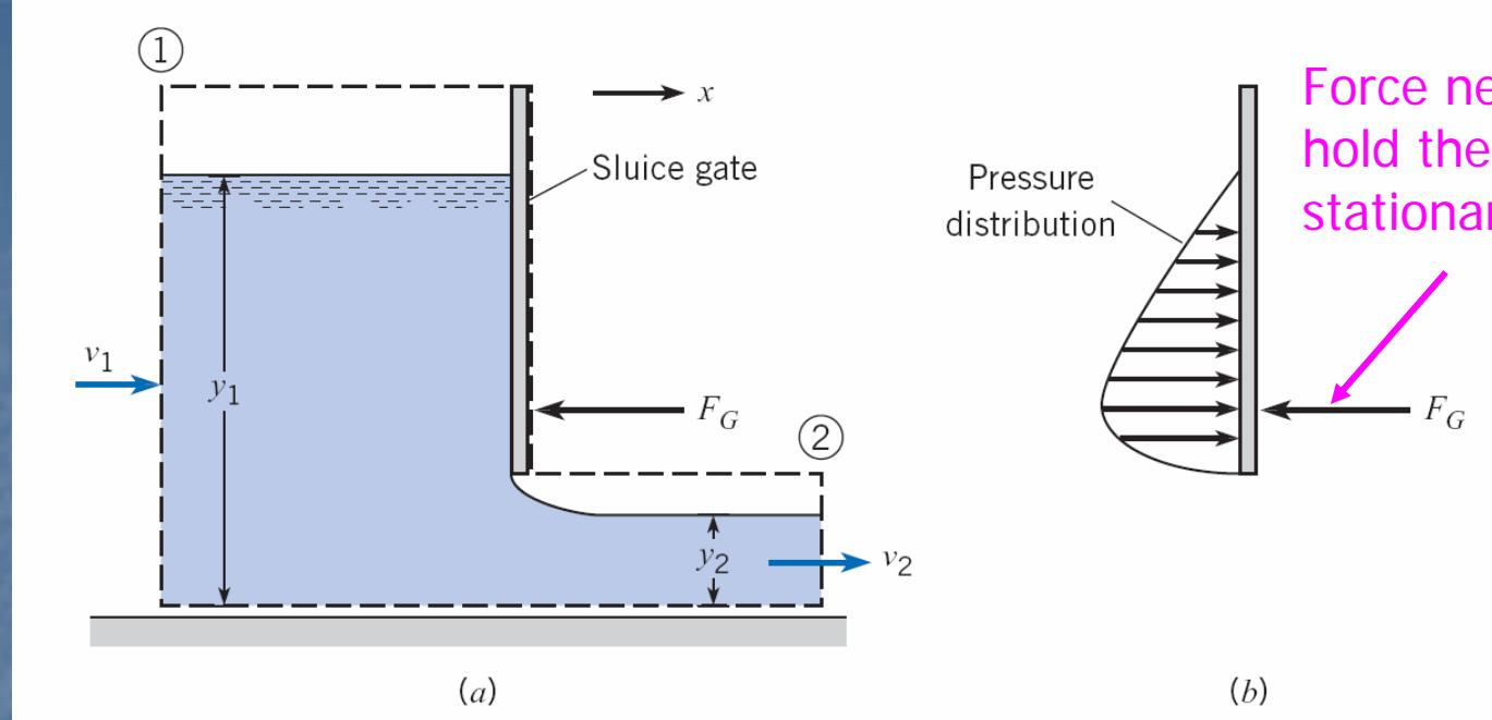
From the force diagram,  $\sum F_x = \bar{p}A_1 - \bar{p}A_2 - F_G - F_{shear}$
