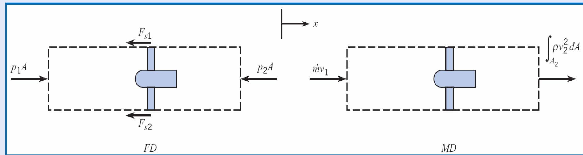
Given:  $v_1 = 30 \text{ m/s}$ ,  $p_1 = 1.5 \text{ kPa gauge}$ ,  $p_2 = 1.0 \text{ kPa gauge}$ ,  $\rho_{\text{air}} = 1.0 \text{ kg/m}^3$ ,  $D = 1 \text{ m}$
